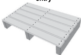
Stringer-class, double-face non-reversible, 2-way entry, 3 bottom runners
