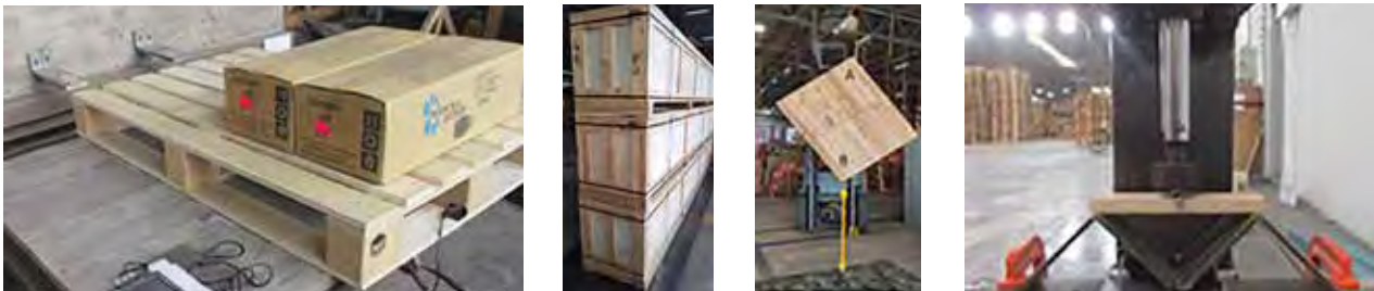
Pictures from left to right: incline impact test, stacking test, drop test and compression test.
