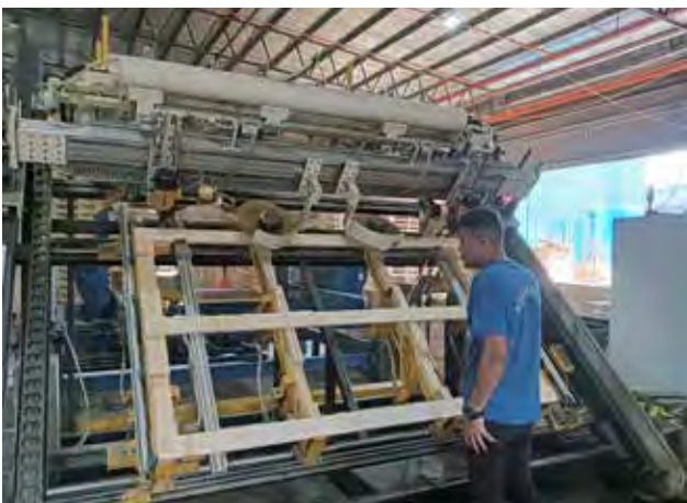
Auto nailer for wooden pallet assembly with stacking station
